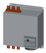
SIRIUS soft starter Values at 690 V, 40 °C standard: 551 A, 560 kW Inside-delta: only up to 600 V 400-690 V AC, 230 V AC Screw terminals !!! Phased-out product !!! Successor is SIRIUS 3RW5, Preferred successor type is >>3RW5548-6HA16<<
