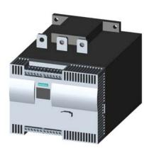
SIRIUS soft starter Values at 500 V, 40 °C standard: 356 A, 250 kW Inside-delta: 617 A, 450 kW 400-600 V AC, 230 V AC Screw terminals !!! Phased-out product !!! Successor is SIRIUS 3RW5, Preferred successor type is >>3RW5546-6HA16<<
