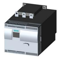
SIRIUS soft starter Values at 400 V, 40 °C standard: 162 A, 90 kW Inside-delta: 281 A, 160 kW 200-460 V AC, 230 V AC Screw terminals !!! Phased-out product !!! Successor is SIRIUS 3RW5, Preferred successor type is >>3RW5536-6HA14<<
